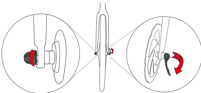
With the lever open, the nut is used to both loosen and pre-tighten the mechanism.
