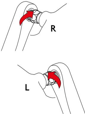
Using finger & thumb (and later a 15mm spanner) attach the pedals onto their crank arms. The **R** pedal will be tightened in a **clockwise** direction.
