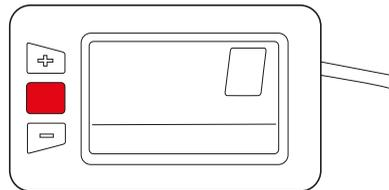
3. **Light Operation:** The front light is connected into the system and powered from the battery. To operate, press and hold the
