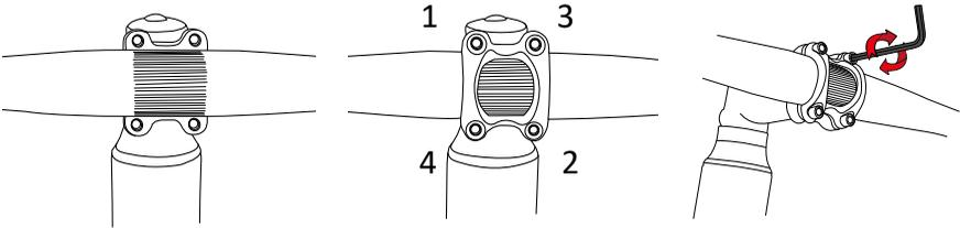
Ensure the handlebars are perpendicular to the front wheel. **Top Tip:** A boarded or tiled floor can help with alignment.
