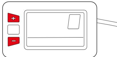
3. **Walk assistance:** Our latest displays offer a low speed “cruise” setting, for use when walking alongside your bike. To activate walk assist, **hold down** the - button. After a few seconds the bike will start.
