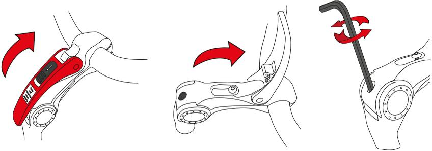
For bikes with a fixed stem, handlebars will be attached to the side of the frame. Avoid releasing the handlebars from the frame until ready to fit them. Leaving them dangling will place strain on the cables.
