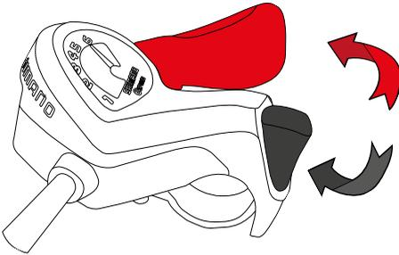
Push lever to lower gear ratio whilst pedalling up-hill
