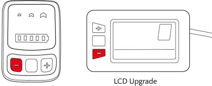
For bikes with a throttle, the red button is depressed and the throttle grip twisted to activate. For safety, when not in use ensure the red button is left out to avoid accidental use of the throttle.
