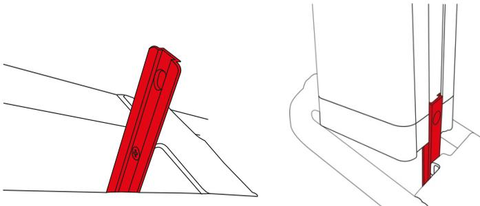
Once fully inserted, turn the key **clockwise** into the **OFF** position to lock the battery in place. The key can then be removed.
