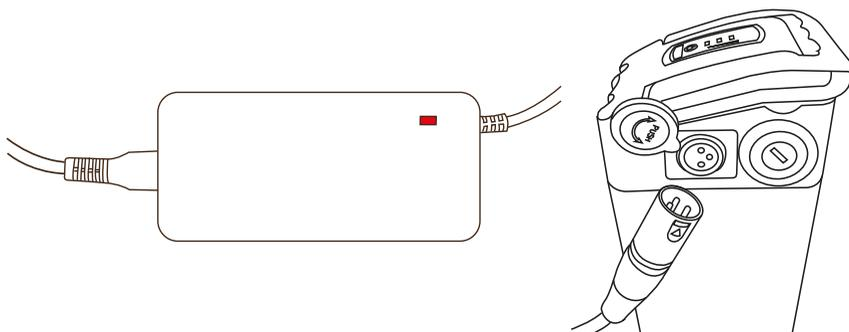
4. **Removing/replacing the battery:** Some of the batteries in our range can be charged in or out of the bike. Push in and turn the key fully anti-clockwise to unlock the battery from the bike. Take care putting the battery back into the bike.
