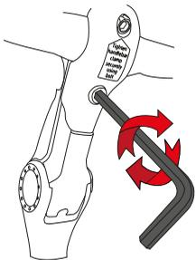
If the handlebars are not holding firm under pressure, the grip may also need tightening. This can be achieved by tightening the bolt underneath the front of the adjuster clamp.
